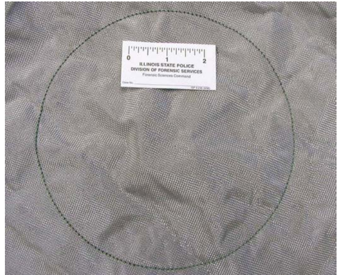
FIG. 5—Single central seam area of deployed driver side airbag from 1996 Dodge Ram pick-up truck.
