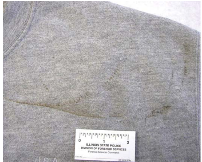
FIG. 4—Single row singe patterns on front upper left quadrant of sweatshirt from suspected driver of crashed 1996 Dodge Ram pick-up truck.
