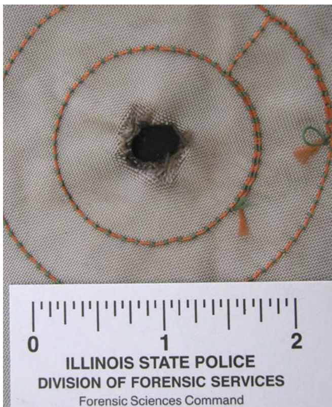
FIG. 7—Single vent hole on back of the deployed driver side airbag from 1996 Dodge Ram pick-up truck.
