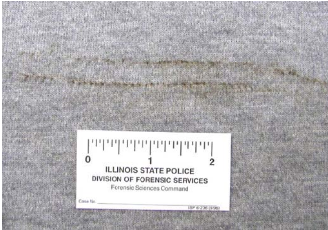
FIG. 2—Double row singe pattern on lower abdominal area of sweatshirt from the suspected driver of crashed 1996 Dodge Ram pick-up truck.
