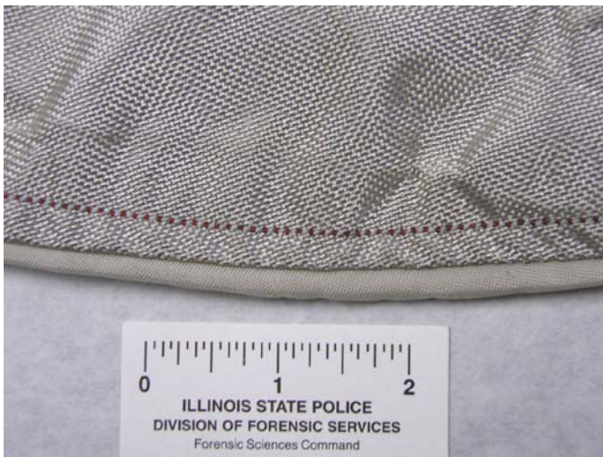
FIG. 3—Double outer seam area of the deployed driver side airbag from 1996 Dodge Ram pick-up truck. Some of the top seam threads are charred and slightly melted.
