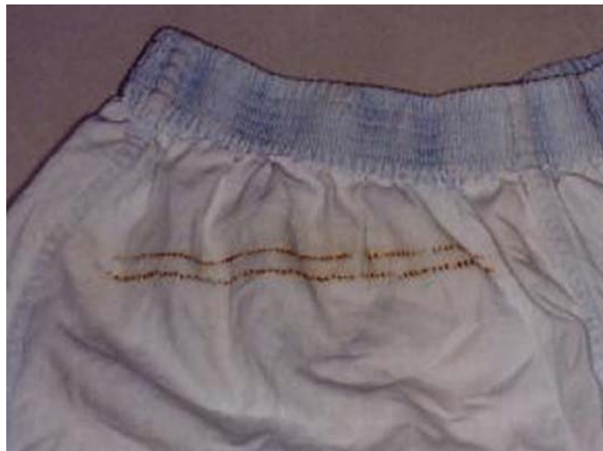
FIG. 1—Singe pattern on shorts from driver of 1991 Lincoln Continental after airbags deployed.
