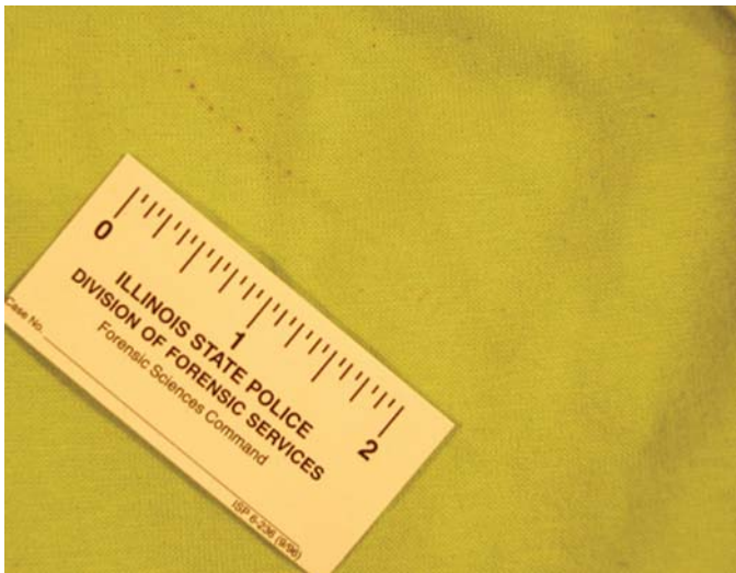
FIG. 9—Straight single row singe pattern on upper left chest area of shirt worn by suspected passenger of crashed 1996 Kia Sephia.
