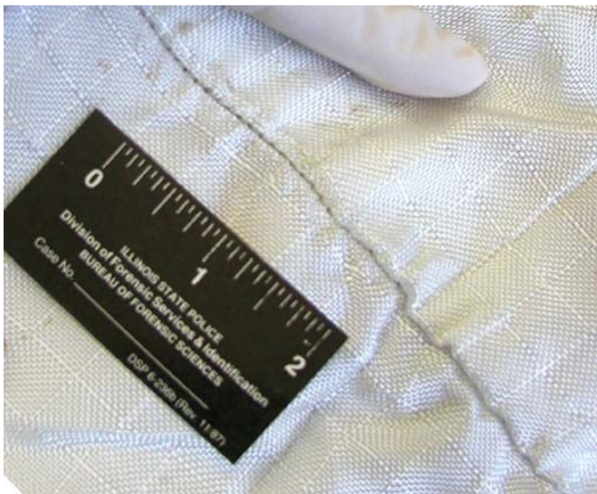
FIG. 11—Straight single seam area on deployed passenger side airbag from 1996 Kia Sephia.
